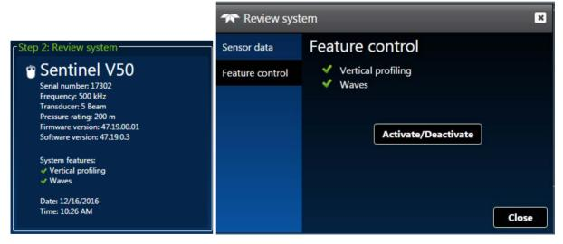
Figure 17. Activating and Deactivating Features
