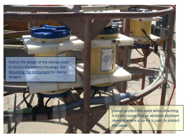
Figure 45. Cables Protected with Abrasion Resistant Sleeving
