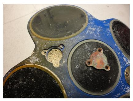
Figure 64. Pressure Sensor Cavity with Sand
