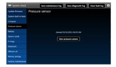
Figure 65. Zero the Pressure Sensor
