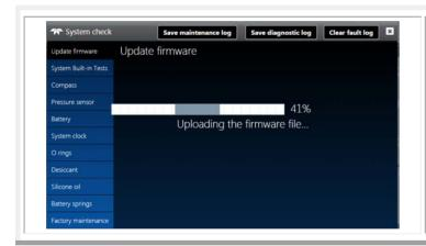
Select **Firmware Upgrade** and then select the Sentinel V Real-Time firmware binary (66.xx.bin) file. Version 66.xx firmware is loaded into the system and then the Sentinel V Real-Time system restarts.
