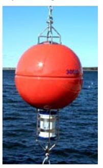
Figure 40. Buoy Mount with External Battery
