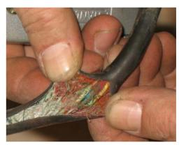
Figure 44. Do not use Zip-Ties Directly on Cables
