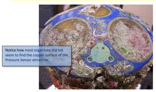
Figure 69. Biofouling on a Sentinel V ADCP
