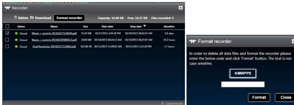
Once the data has been recovered, the recorder can be erased by clicking the **Format recorder** button. Enter the code and then click the **Format** button at the prompt. *Once erased, the data is not recoverable.*
