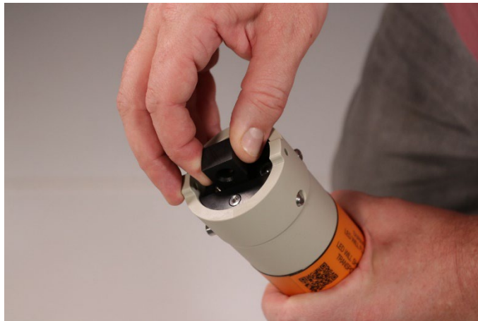
Figure 4-1 Loading the Release Nut into the Release Mechanism
