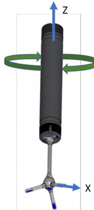
**Figure: Rotate the instrument to verify compass functionality. Clockwise is positive**
