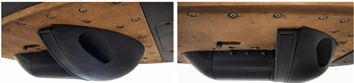
Hull mounted WINGHEAD sonar installation on the DriX Unmanned Surface Vessel (USV)
